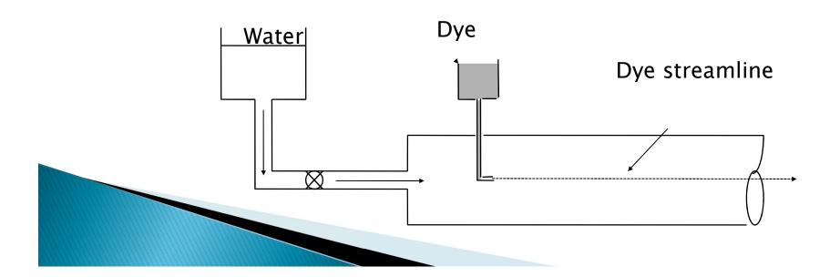
As the velocity of the water was increased, it was found that at a definite velocity the thread of dye became dispersed and the pattern was very erratic. (Turbulent flow)
