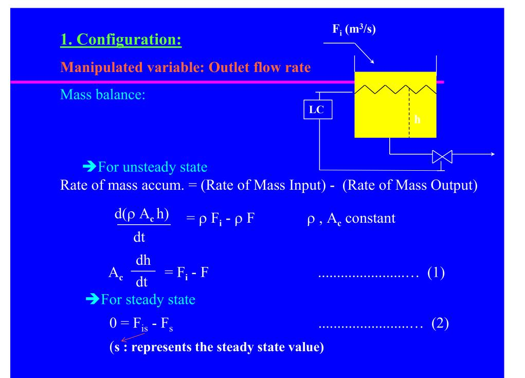
Subtract Equation (2) from Equation (1);  $A_{c} \frac{dh}{dt} = (F_{i} - F_{is}) - (F - F_{s})$
