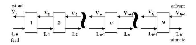
Schematic representation of a multistage countercurrent extraction process
