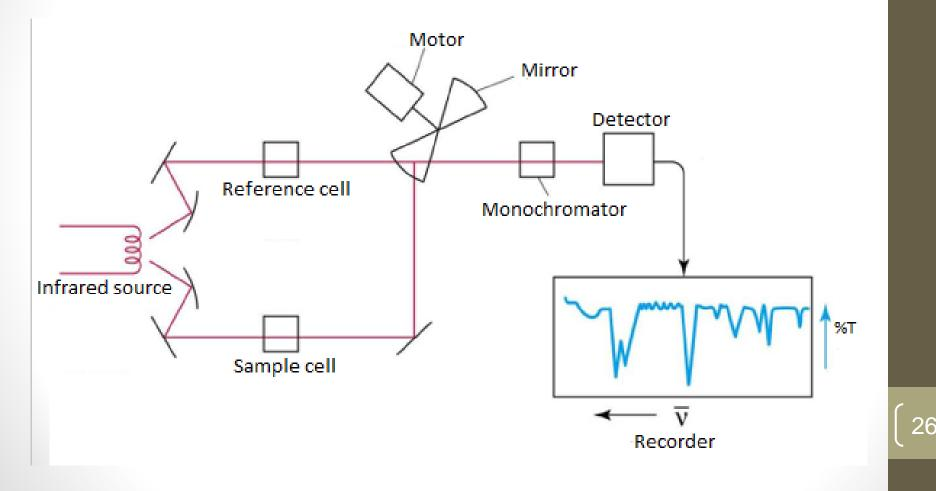
Two types of infrared spectrometers are in common use in the organic laboratory: single beam and double beam. A modern double beam instrument consists of 5 parts, a source of radiation, a photometer, a monochromator, a detector system and a recorder.
