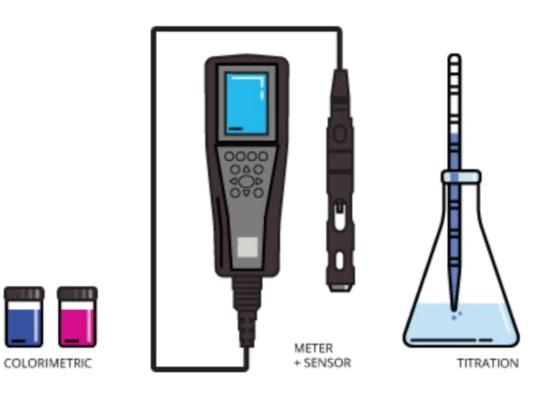
Dissolved oxygen can be measured by colorimetry, a sensor and meter or by titration.
