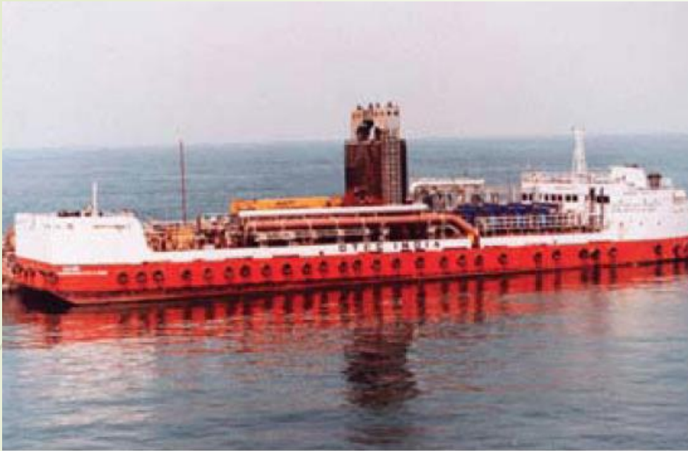
Demonstration of 1 MW OTEC Device Thermo-dynamic Rankine cycle (Saga University, Japan)
