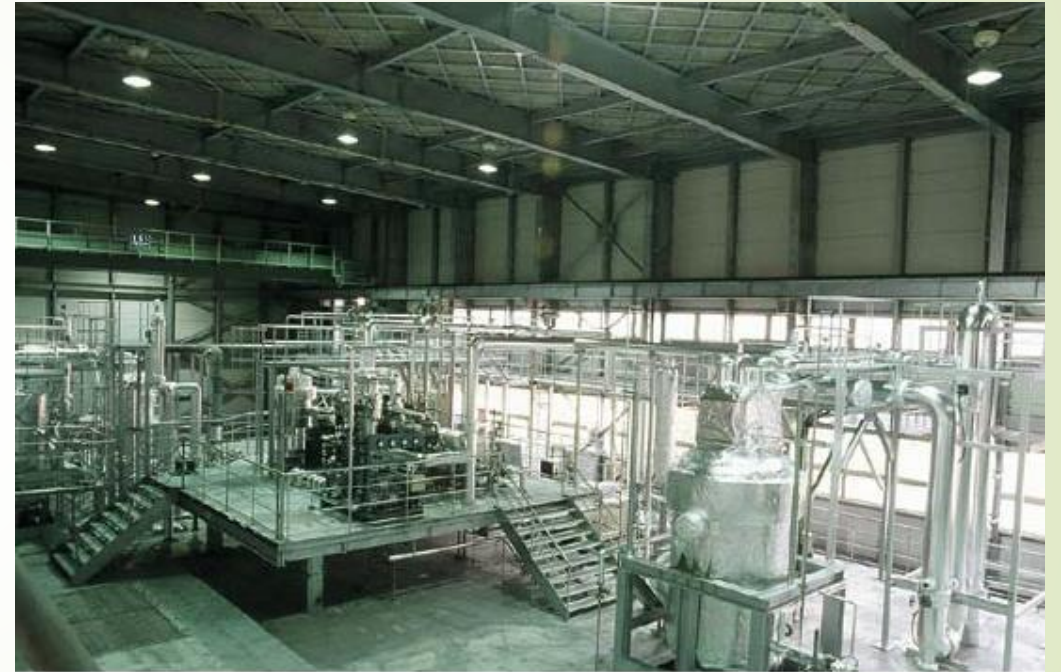
Experimental 30 kW OTEC system (Saga University, Japan)
