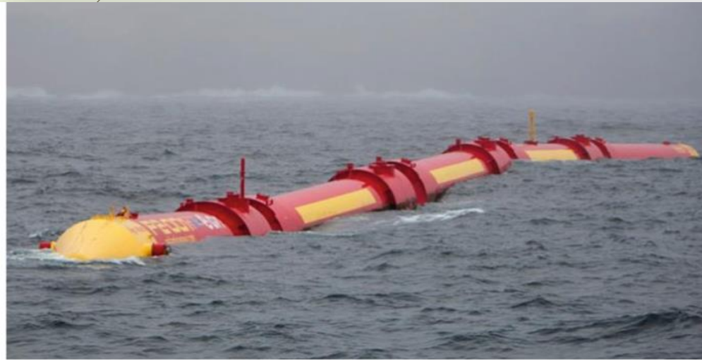
Fig. 9 E.ON P2 Pelamis operating in Orkney July 2011 [27]
