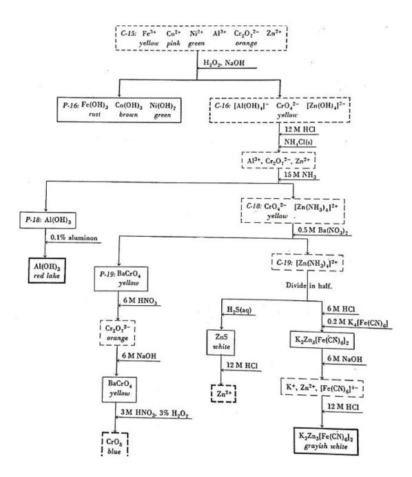
Qualitative analysis flowchart for The Ammonium Sulfide Subgroup 3B
