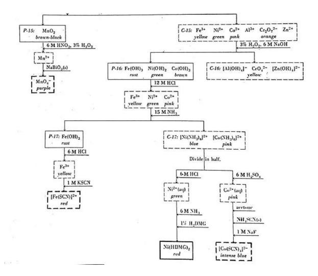
Qualitative analysis flowchart for The Ammonium Sulfide Subgroup 3A
