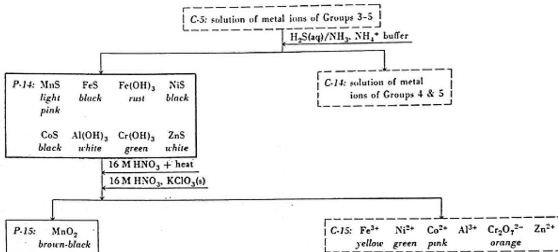
**Qualitative analysis flowchart for The Ammonium Sulfide Group: Precipitation and separation into two subgroups**
