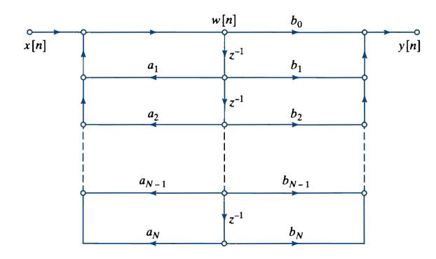
Signal flow graph of direct form II structure for an *N*<sup>th</sup>-order system
