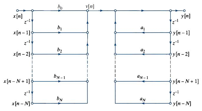
Signal flow graph of direct form I structure for an N<sup>th</sup>-order system
