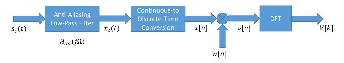
Processing steps in the Discrete-Time Fourier analysis of a continuous-time signal
