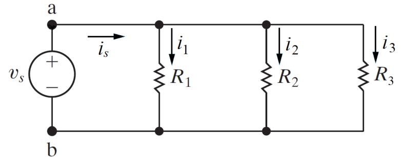
$$i_{S} = \frac{v_{S}}{R_{1}} + \frac{v_{S}}{R_{2}} + \frac{v_{S}}{R_{3}}$$
