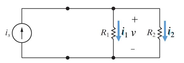
$$i_{s} = i_{1} + i_{2} = \frac{v}{R_{1}} + \frac{v}{R_{2}}$$
