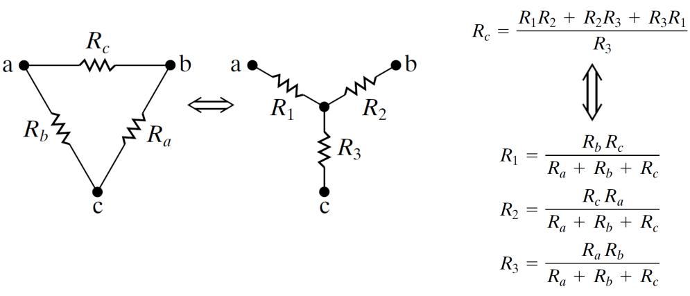
$R_a = \frac{R_1 R_2 + R_2 R_3 + R_3 R_1}{R_1}$
