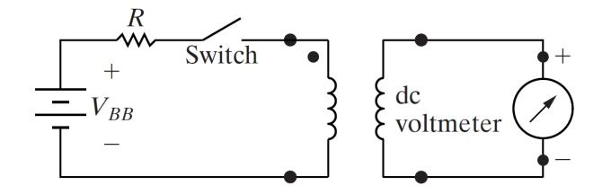
Determining polarity marks experimentally
