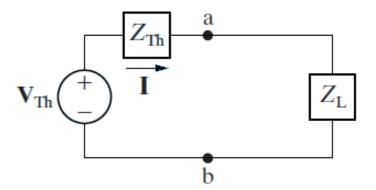
If the Thevenin voltage is expressed in terms of its rms amplitude, the maximum average power delivered to the load is
