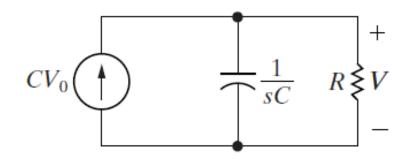
$$\frac{V}{R} + sCV = CV_0 \implies V = \frac{V_0}{s + \left(\frac{1}{RC}\right)} \longrightarrow v = V_0 e^{-t/(RC)} u(t)$$
