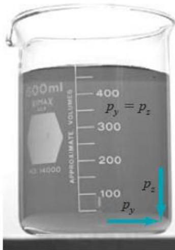
**Figure 3.4. The pressure at a point in a fluid at rest is independent of direction.**
