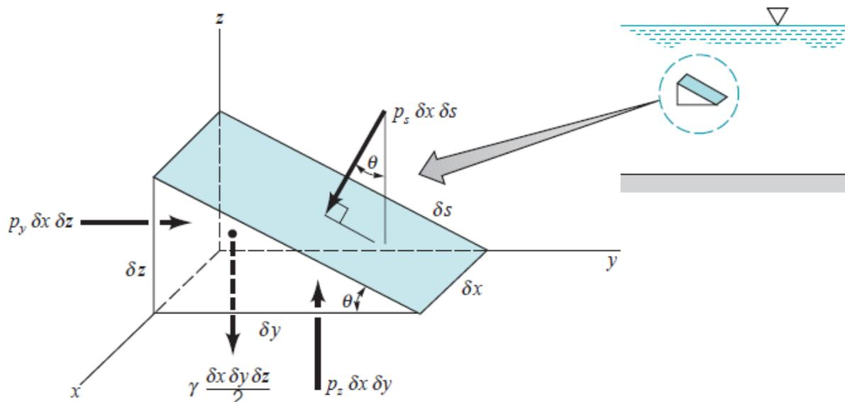
**Figure 3.3. Forces on an arbitrary wedge-shaped element of fluid. Where  $P_s$ ,  $P_y$ , and  $P_z$ , are the average pressures on the faces, and  $\gamma$  and  $\rho$  are the fluid specific weight and density, respectively, and  $a_y$ ,  $a_z$  are the accelerations.**
