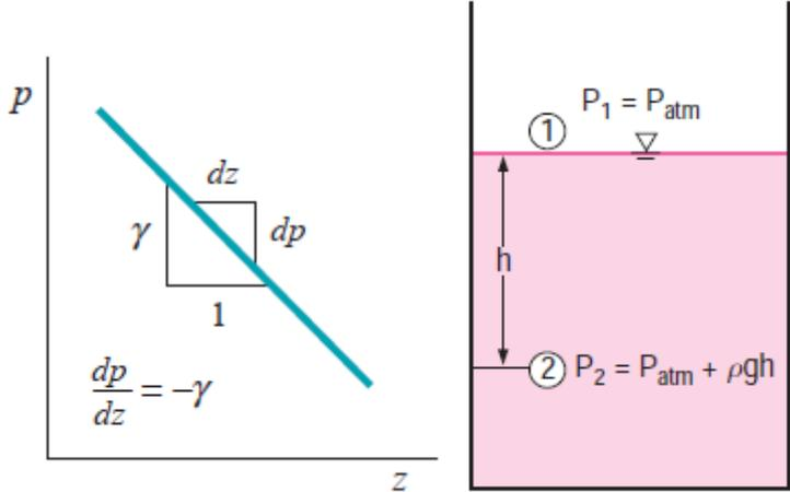
**Figure 3.6. For liquids or gases at rest, the pressure gradient in the vertical direction at any point in a fluid depends only on the specific weight of the fluid at that point.**
