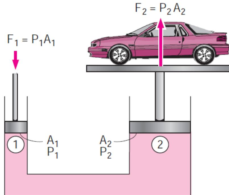
**Figure 3.9. Lifting of a large weight by a small force by the application of Pascal’s law.**
