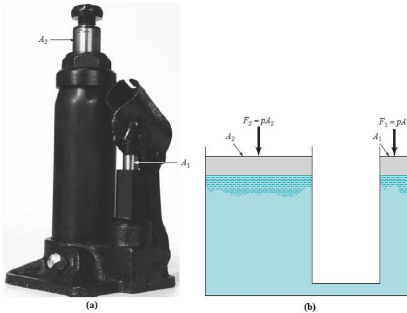
**Figure 3.10. (a) Hydraulic jack, (b) Transmission of fluid pressure.**
