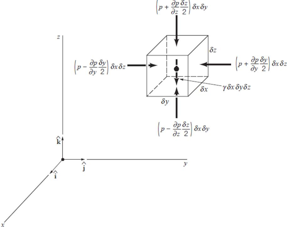
**Figure 3.5. Surface and body forces acting on small fluid element.**
