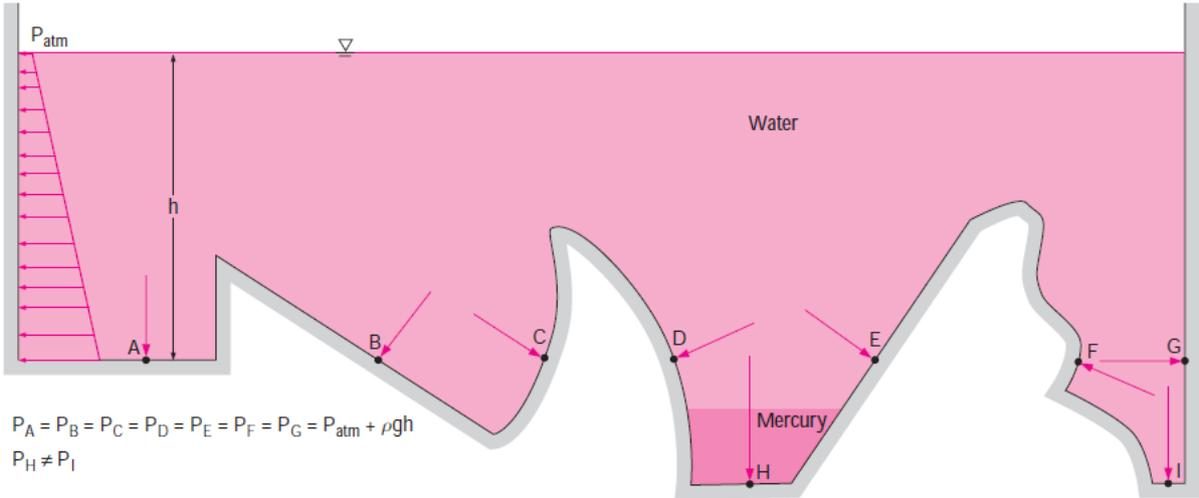
**Figure 3.7. The pressure is the same at all points on a horizontal plane in a given fluid regardless of geometry, provided that the points are interconnected by the same fluid.**
