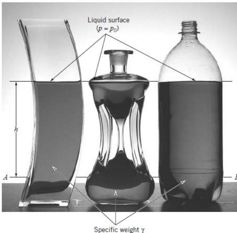
**Figure 3.8. Fluid pressure in containers of arbitrary shape.**
