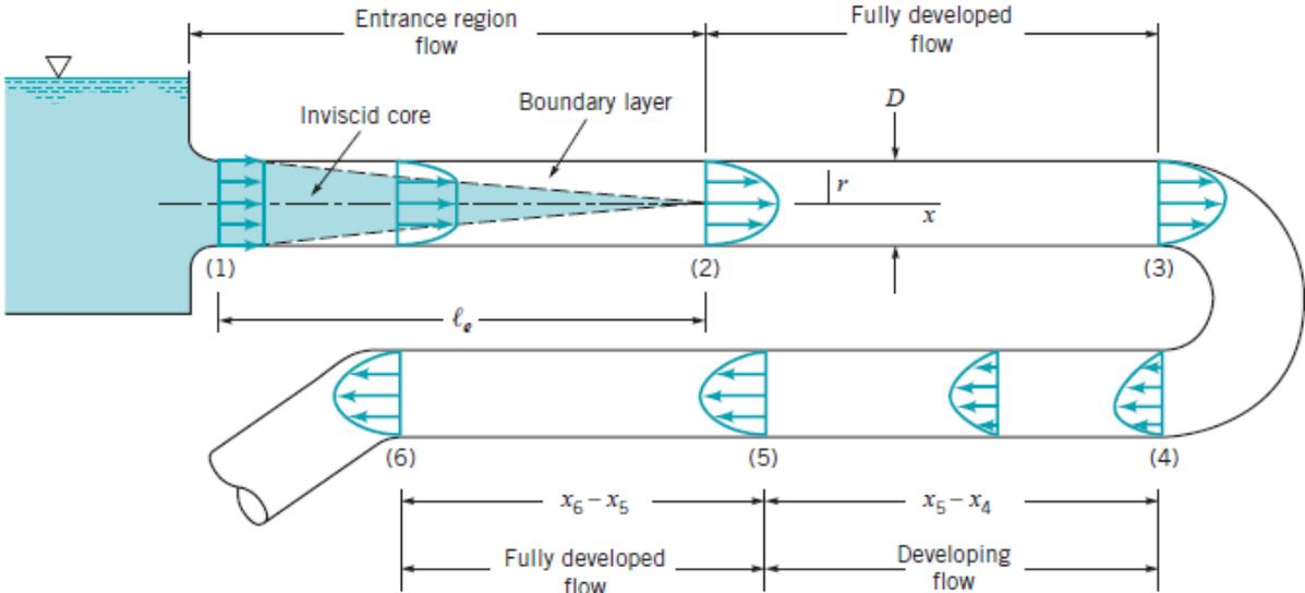
**Figure 5.6. Entrance region, developing flow, and fully developed flow in a pipe system.**
