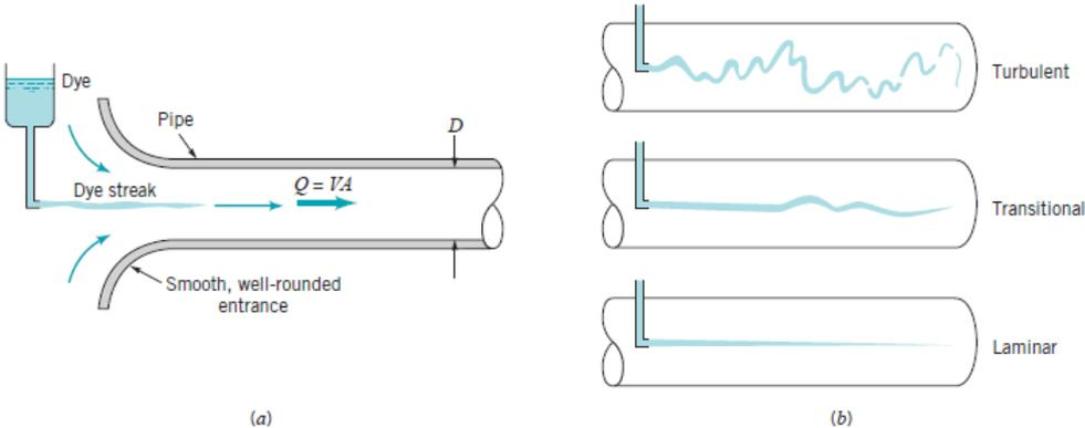
**Figure 5.4. (a) Experiment to illustrate type of flow. (b) Typical dye streaks.**
