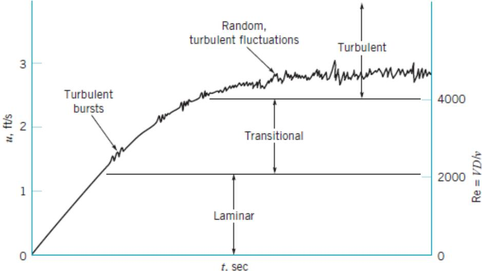
**Figure 5.10. Transition from laminar to turbulent flow in a pipe.**
