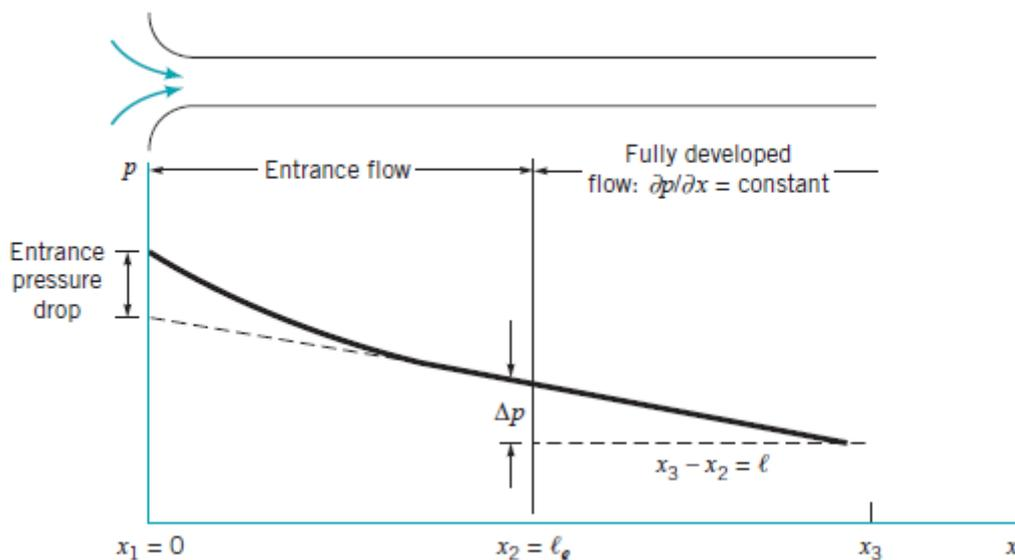
**Figure 5.7. Pressure distribution along a horizontal pipe.**
