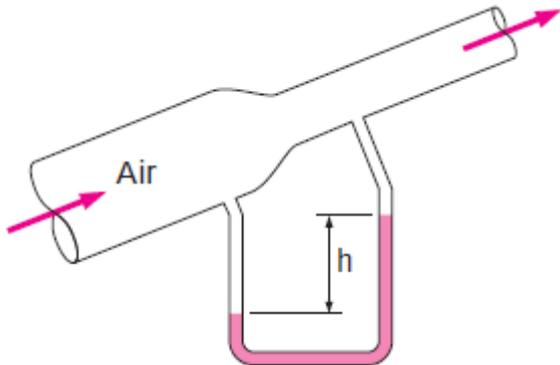
**Solution:** We take points 1 and 2 at the lower and upper connection points, respectively, of the two arms of the manometer, and take the lower connection point as the reference level. Noting that the effect of elevation on the pressure change of a gas is negligible, the application of the Bernoulli equation between points 1 and 2 gives
