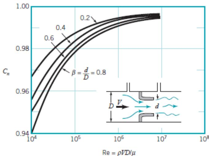
**Figure 5.26. Nozzle meter discharge coefficient**
