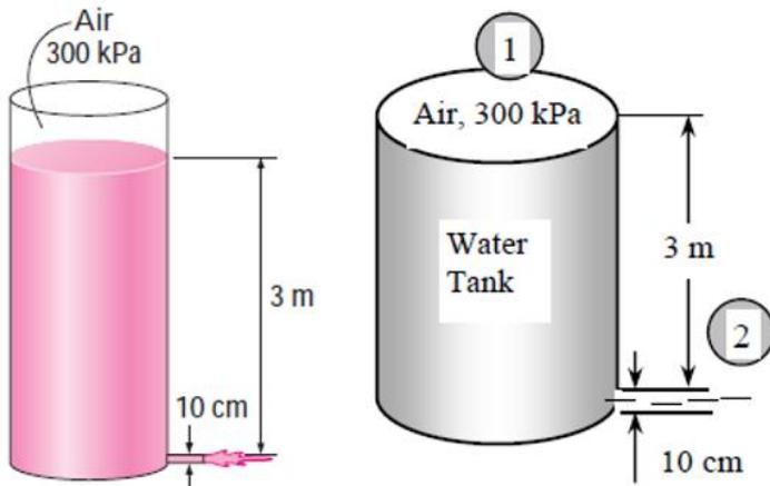
**Solution:** We take point 1 at the free surface of the tank, and point 2 at the exit of orifice, which is also taken to be the reference level ( $z_2 = 0$ ). Noting that the fluid velocity at the free surface is very low ( $V_1 \cong 0$ ) and water discharges into the atmosphere (and thus  $P_2 = P_{\text{atm}}$ ), the Bernoulli equation simplifies to
