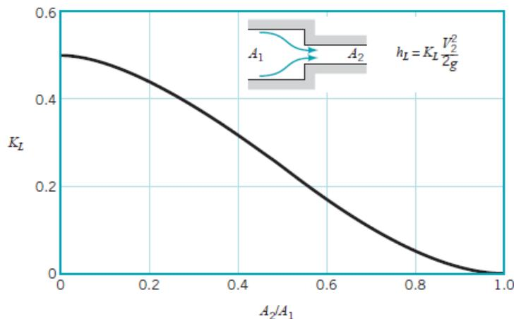
**Figure 5.20. Loss coefficient for a sudden contraction**
