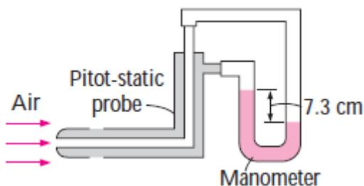
**Solution:** We take point 1 on the side of the probe where the entrance is parallel to flow and is connected to the static arm of the Pitot-static probe, and point 2 at the tip of the probe where the entrance is normal to flow and is connected to the dynamic arm of the Pitot-static probe. Noting that point 2 is a stagnation point and thus  $V_2 = 0$  and  $z_1 = z_2$ , the application of the Bernoulli equation between points 1 and 2 gives
