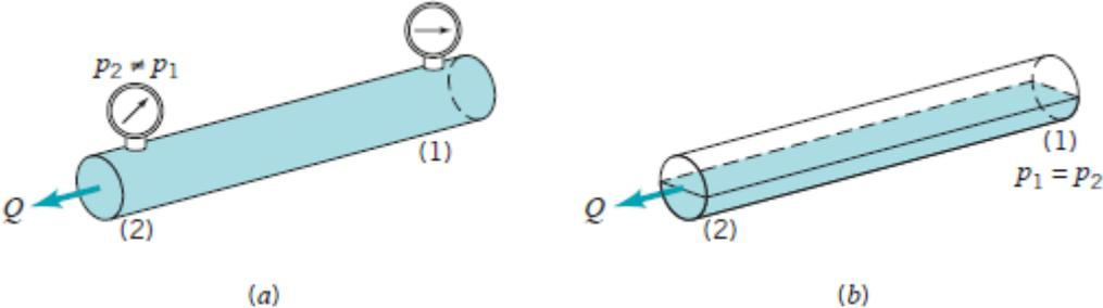
**Figure 5.3. (a) Pipe flow. (b) Open-channel flow.**
