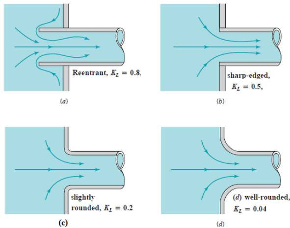
**Figure 5.18. Entrance flow conditions and loss coefficient**
