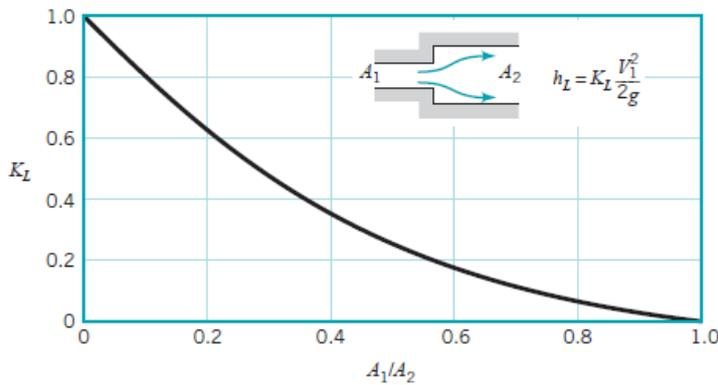
**Figure 5.21. Loss coefficient for a sudden expansion**
