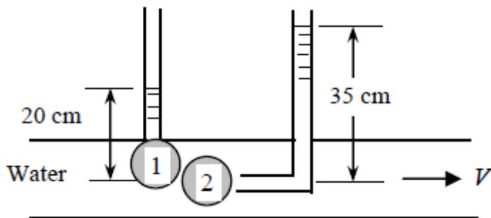
$$\frac{P_1}{\rho g} + \frac{V_1^2}{2g} + z_1 = \frac{P_2}{\rho g} + \frac{V_2^2}{2g} + z_2 \rightarrow \frac{V_1^2}{2g} = \frac{P_2 - P_1}{\rho g}$$
