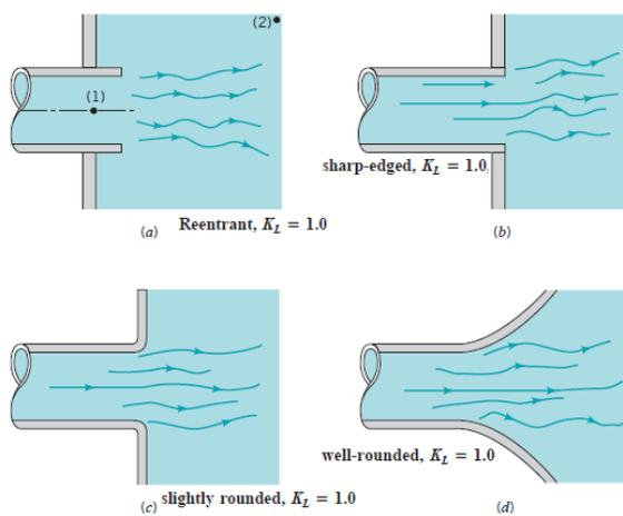
**Figure 5.19. Exit flow conditions and loss coefficient.**
