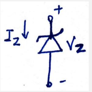
Common zener diode voltage ratings are between 1.8V and 200V
