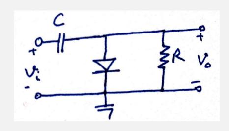
A diode and capacitor can be combined to "clamp" an AC signal to a specific DC level.
