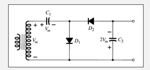
This half-wave voltage doubler's output can be calculated using:
