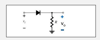
The diode in a series clipper "clips" any voltage that does not forward bias it:
