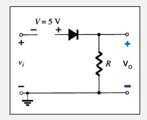
Adding a DC source in series with the clipping diode changes the effective forward bias of the diode.
