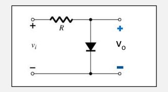
The diode in a parallel clipper circuit "clips" any voltage that forward biases it.
