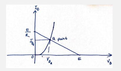
The point where the load line and the characteristic curve intersect is the Q-point, which identifies  $I_D$  and  $V_D$  for a particular diode in a given circuit.
