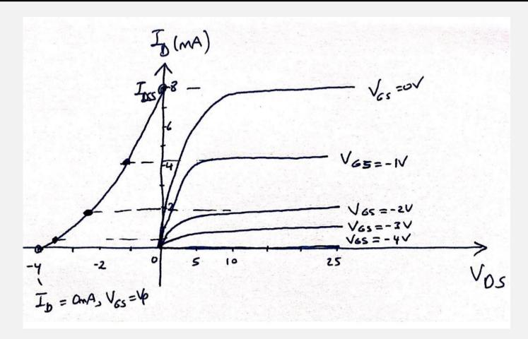
This graph shows the value of  $I_D$  for a given value of  $V_{GS}$ .
