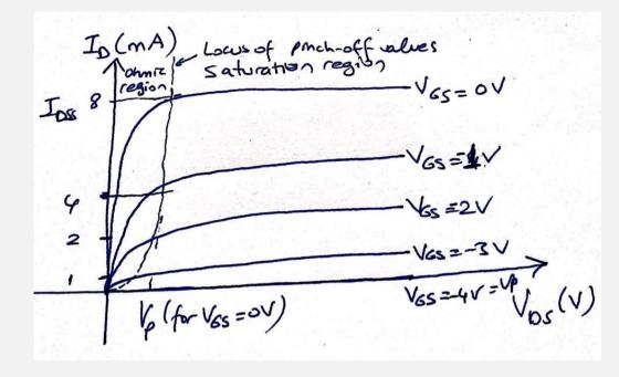
Note that at high levels of  $V_{DS}$  the JFET reaches a breakdown situation.  $I_D$  increases uncontrollably if  $V_{DS} > V_{DSmax}$ , and the JFET is likely destroyed.
