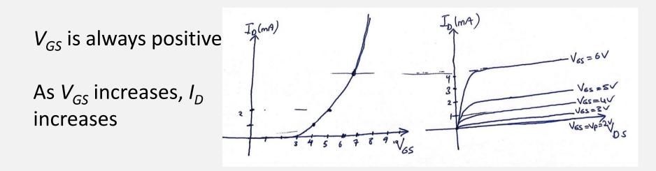
As  $V_{GS}$  is kept constant and  $V_{DS}$  is increased, then  $I_D$  saturates  $(I_{DSS})$  and the saturation level  $(V_{DSSat})$  is reached
