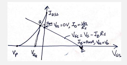
The Q-point is located where the line intersects the transfer curve
