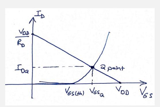
Using the value of I<sub>D</sub> at the Q-point, solve for the other variables in the circuit
