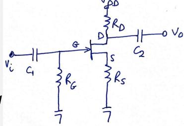
$$V_{DS} = V_{DD} - I_D (R_S + R_D)$$
