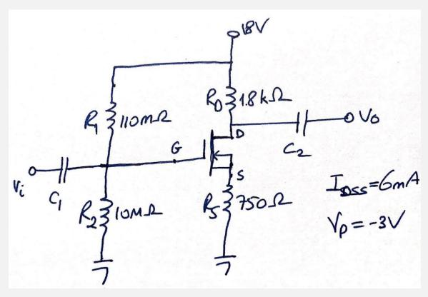
Depletion-type MOSFET bias circuits are similar to those used to bias JFETs. The only difference is that D-type MOSFETs can operate with positive values of  $V_{GS}$  and with  $I_D$  values that exceed  $I_{DSS}$ .
