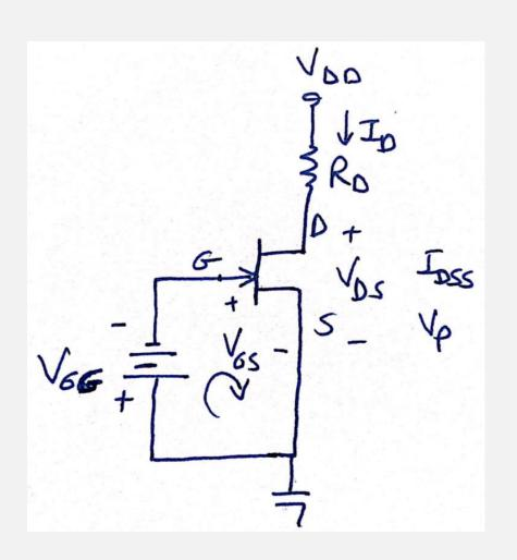
$$egin{aligned} V_{DS} &= V_{DD} - I_D R_D \ V_S &= 0 \ V \ V_C &= V_{DS} \ V &= V_{GS} \ V_{GS} &= -V_{GG} \end{aligned}$$
