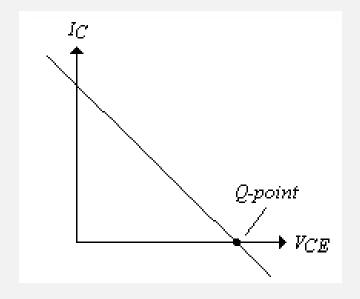
The Q-point is at 0 V on the load line, so that the AC signal can only swing for one-half cycle.
