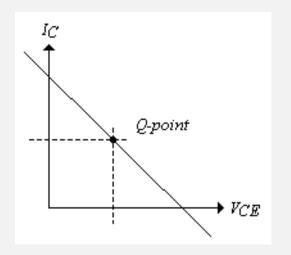
Remember that the DC load line indicates the minimum & maximum output voltage and current allowed by the DC power supply.
