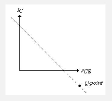
The output of the class C conducts for less than 180° of the AC cycle. The Q-point is below cutoff.
