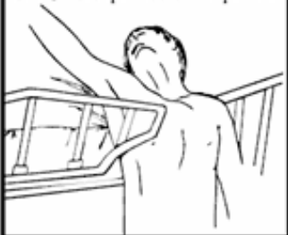
Zone 5 - Entrapment between split rails
