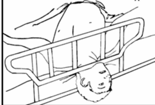
Zone 2 - Entrapment between top of compressed mattress to bottom of rail, between rail and supports
