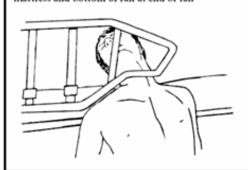
Zone 4 - Entrapment between top of compressed mattress and bottom of rail at end of rail
