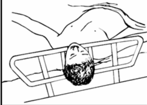
Zone 1 - Entrapment within rail
