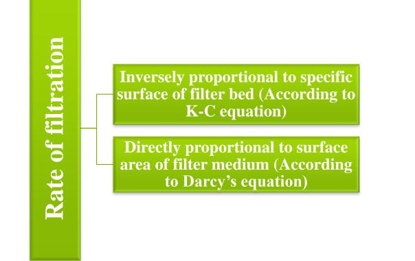
Rate can be increased either using large filter or connecting a number of small units in parallel. Filter press works on principle of connecting units in parallel.
