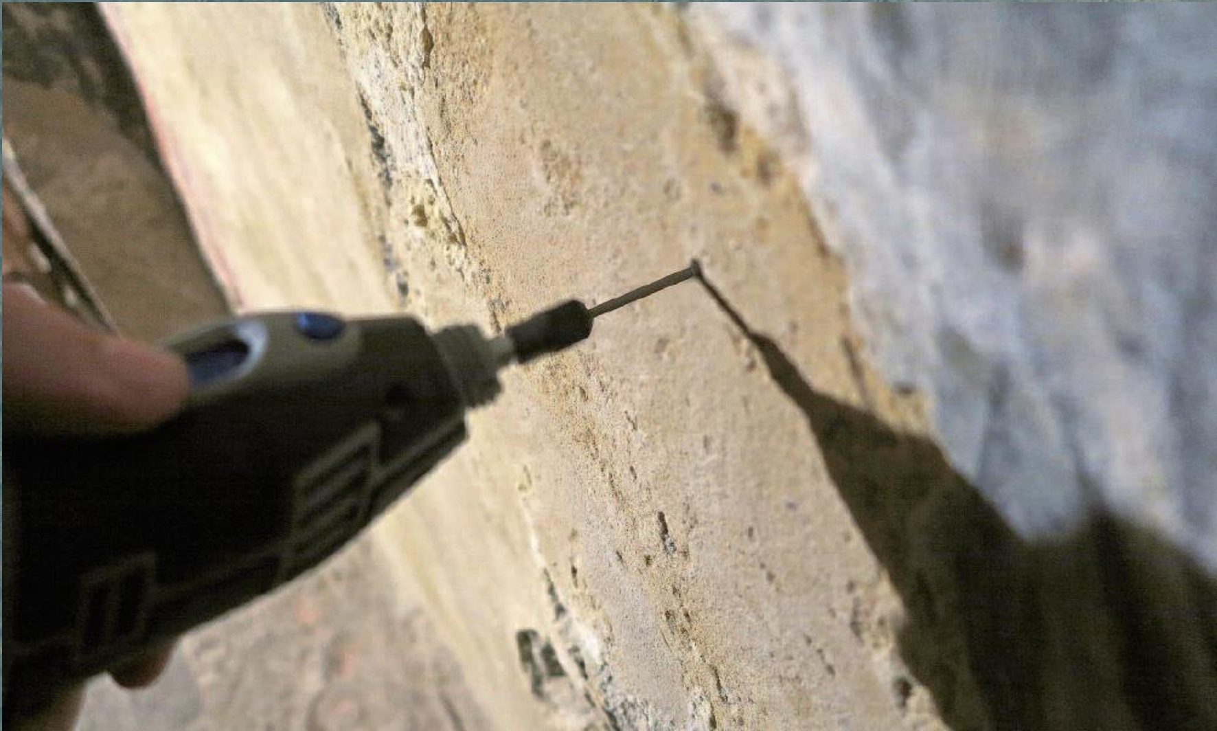
Drill core sampling of a restoration render, Chapel of Notre Dame d'Entrevignes, Sigale (France), 16th century; Photo: 2013, CICRP (Jean-Marc Vallet); Weyer, E. (ed.), (2015), EwaGlos:European Illustrated Glossary Of Conservation Terms For Wall Paintings And Architectural Surfaces, Petersberg: Hornemann Institute; 268.
