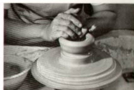
FIGURE 8. The wall is squeezed to broaden and begin to shape the bowl.
