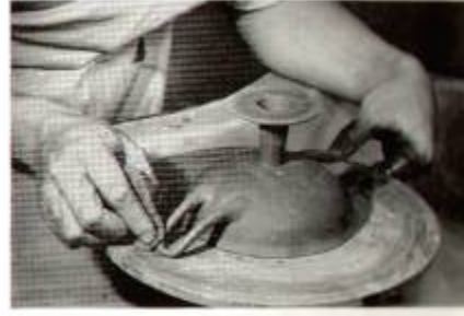
FIGURE 56. A wet sponge is used to smooth the joints on the surface.
