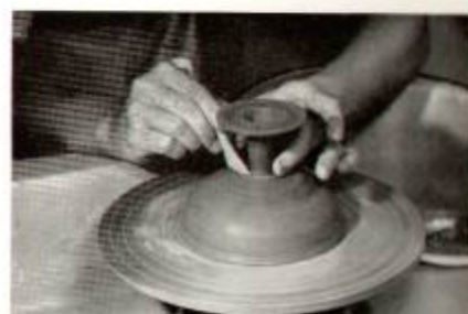
FIGURE 48. More wet clay is applied around the joint.
