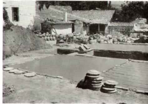
FIGURE 77. Modern Attic clay settling basins. (p. 3)
