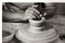
FIGURE 8. The wall is squared to broaden and begin to shape the bowl.
