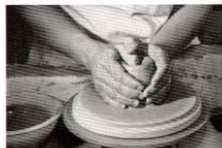
FIGURE 6. When the clay runs true without wobble, a central hole is started.
