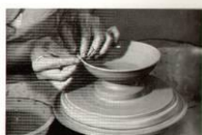
FIGURE 12. A wet leather strip finishes the lip.
