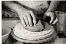
FIGURE 2. The clay is repeatedly wedged by stacking the lower half on the upper.
