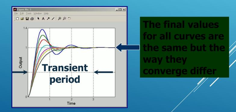
Transient response is the evolution of the signals in a control system until the final behavior is reached.
