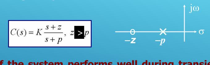
If the system performs well during transient period but poor during steady state, use a lag compensator to improve the steady state characteristics. Lag compensator increases the loop gain without modifying the locations of the dominant CL poles significantly. This is true as long as you locate *p* and *z* close to each other, furthermore, both are located close to origin. **Design based on Root Locus** Lag Compensation
