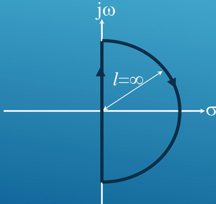
**Since the radius is  $\infty$ , the interior of this closed contour contains every unstable zero or pole of the open loop transfer function  $G(s)H(s)$ , and we can use the theorems of complex mathematics for our goals.**
