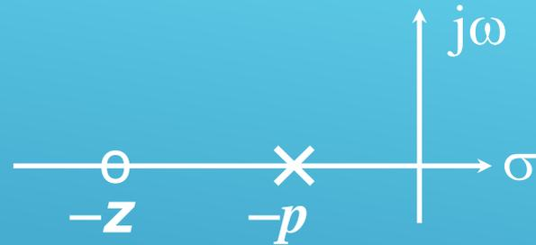
If the system performs well during transient period but poor during steady state, use a lag compensator to improve the steady state characteristics. Lag compensator increases the loop gain without modifying the locations of the dominant CL poles significantly. This is true as long as you locate  $p$  and  $z$  close to each other, furthermore, both are located close to origin.
