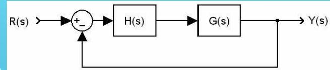
$$G(s) = \frac{N(s)}{D(s)} = \frac{N(s)}{D'(s)(s + \alpha)} \quad \text{and} \quad H(s) = \frac{A(s)}{B(s)} = \frac{A'(s)(s + \alpha)}{B(s)}$$
