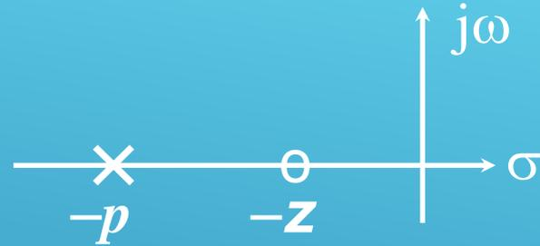
Calculate the angle deficiency ( $\phi$ ) at given locations, which are the desired CL pole locations, and then locate  $p$  and  $z$  to provide the  $-\phi$  to satisfy angle condition. Then calculate  $K$  from the magnitude condition.
