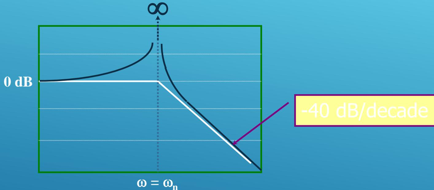
$$G(s) = \frac{\omega_n^2}{s^2 + \omega_n^2} \quad |G(j\omega)| = \frac{1}{\left|1 - \left(\frac{\omega}{\omega_n}\right)^2\right|}$$
