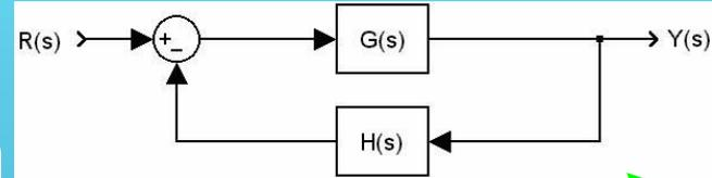
$$G(s) = \frac{N(s)}{D(s)} = \frac{N(s)}{D'(s)(s + \alpha)} \quad \text{and} \quad H(s) = \frac{A(s)}{B(s)} = \frac{A'(s)(s + \alpha)}{B(s)}$$
