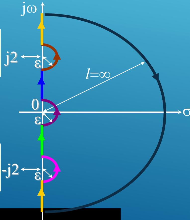
Detour around every  $j\omega$  axis pole by adding a semicircle of infinitesimal radius  $\varepsilon$ !
