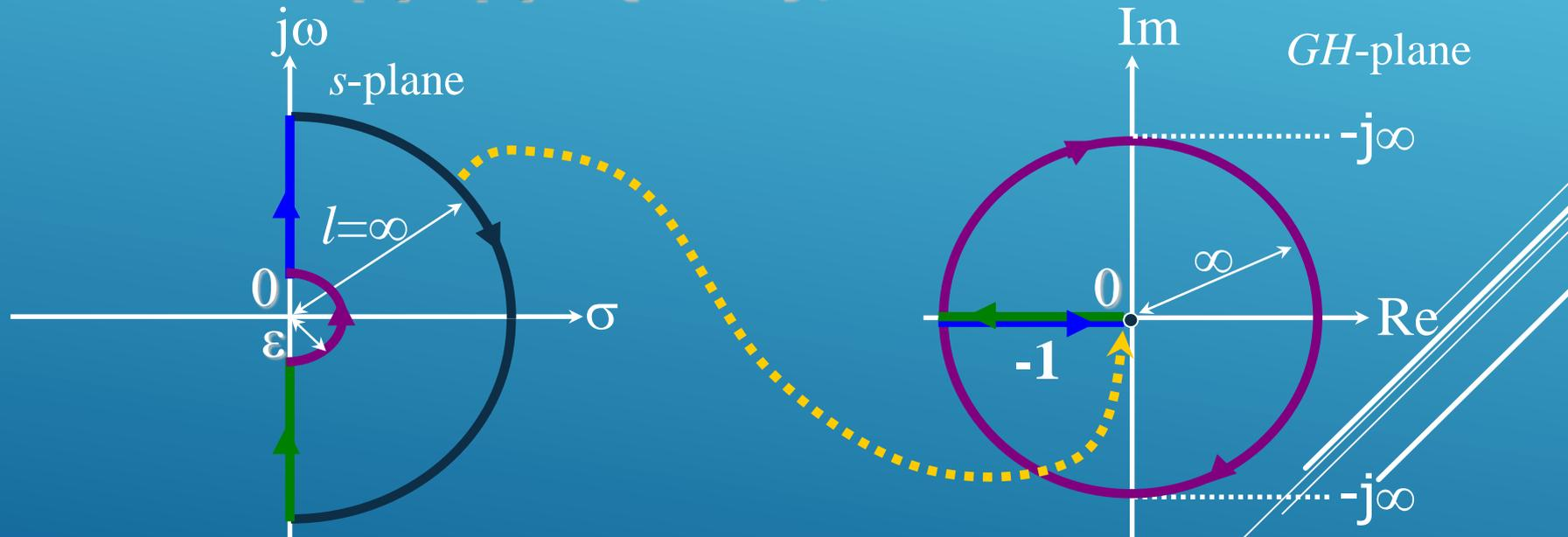
**Locus passes through  $-1+j0$  point, i.e. the closed loop poles are located on the  $j\omega$  axis,  $s^2+K=0$  !**
