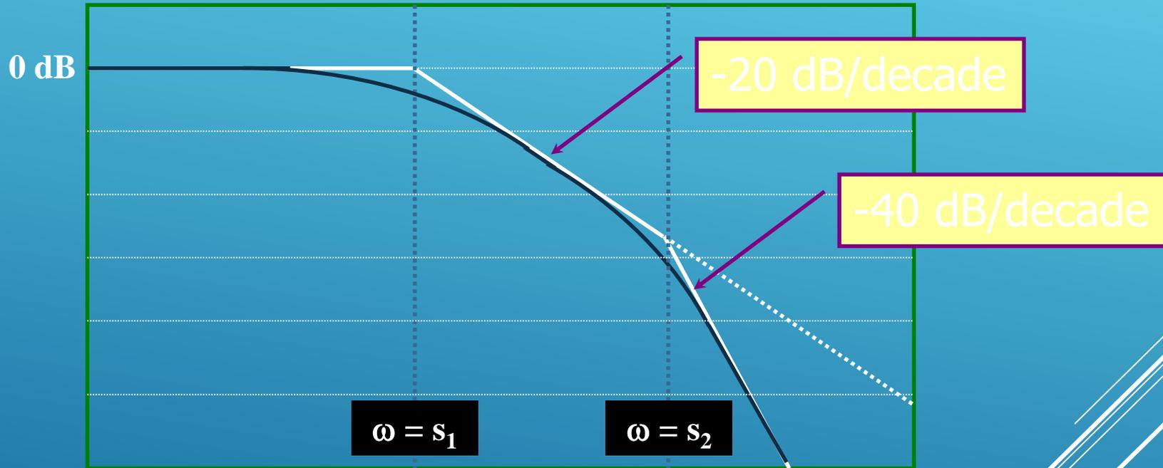
$$G(s) = \frac{\omega_n^2}{s^2 + 2\zeta\omega_n s + \omega_n^2} = \frac{\omega_n^2}{(s - s_1)(s - s_2)}$$
