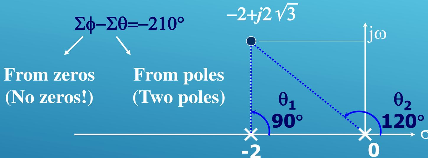
**Compensator must provide  $30^\circ$  to satisfy the angle condition. Remember the p & z configuration of the lead compensator.**
