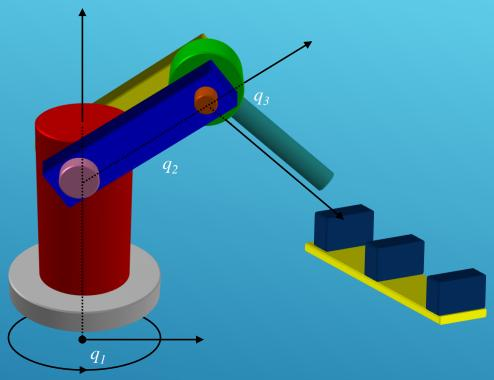
If this robot grasps a load, some parameters seen in its dynamical representation change. If a position control application is being executed, the controller must take this change into account to maintain precision.
