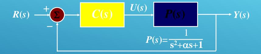
If a controller C(s) meets the design specifications for every  $\alpha$  in a known range  $\alpha_{min} \le \alpha \le \alpha_{max}$  then the controller is a robust controller, and the control system is robust against variations in  $\alpha$ .
