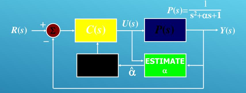
If  $\alpha$  is unknown, we can devise an estimation scheme; and based on the estimated value  $\alpha$ , we can perform the design, and operate the controller in the loop.
