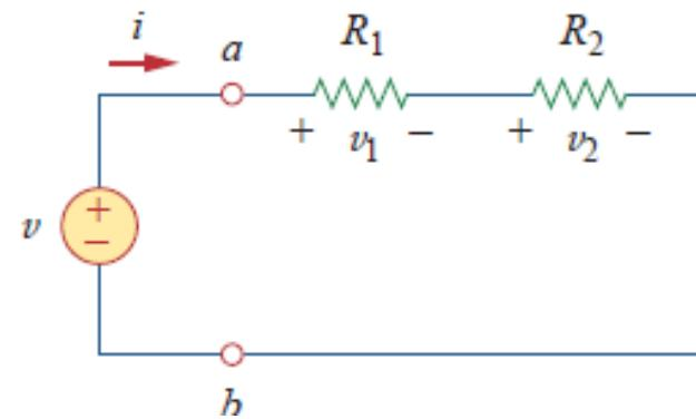
$$v_1 = iR_1, \quad v_2 = iR_2$$
