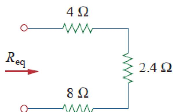
$$R_{eq} = 4 \Omega + 2.4 \Omega + 8 \Omega = 14.4 \Omega$$
