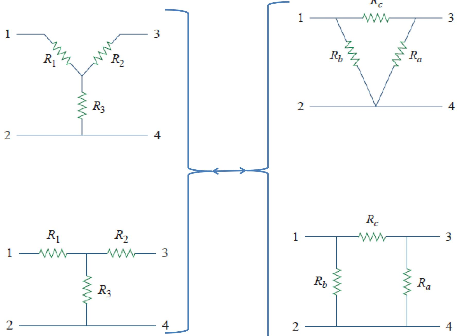
$$R_1 = \frac{R_b R_c}{R_a + R_b + R_c}$$
