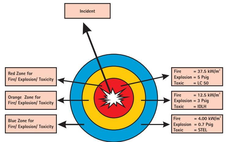
Fig-3 Limits of hazard zones for fire, explosion and toxic release
