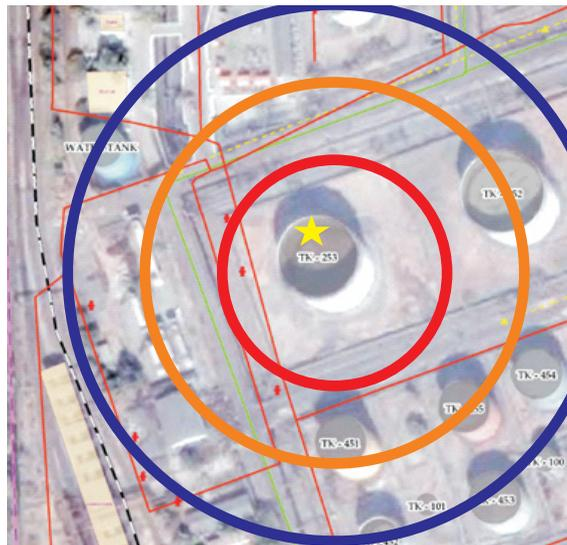
Fig-4 An example how to show the consequence due to fire or explosion
