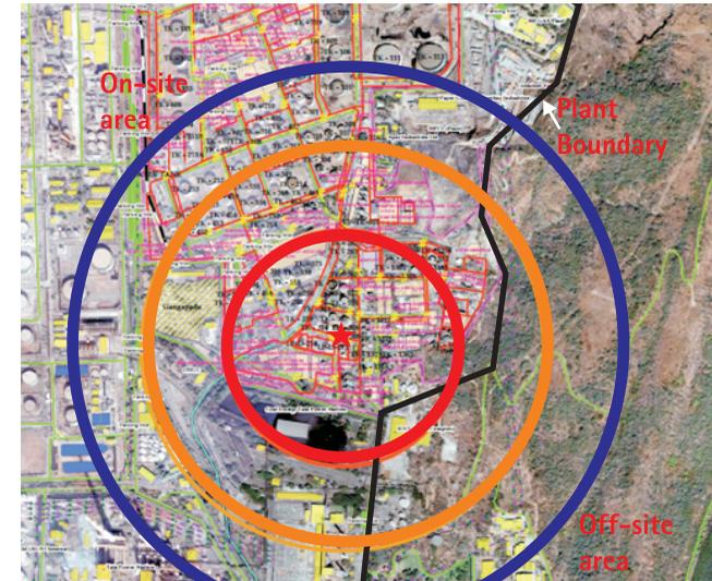
Fig-5 An example how to show the consequence due to fire or explosion to highlight on-site and off-site scenarios
