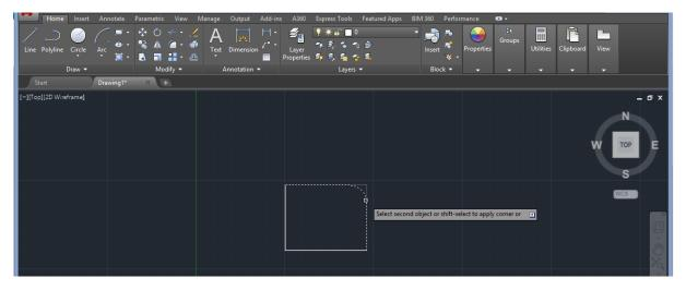
Chamfer: Bevels the edges of objects.
