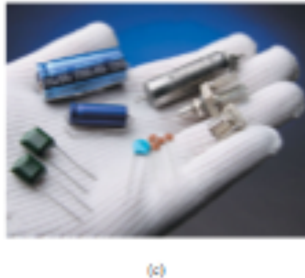
FIGURE 17-19 Capacitors: diagrams of (a) parallel plate, (b) cylindrical (rolled up parallel plate). (c) Photo of some real capacitors.
