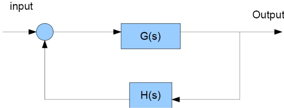
A closed loop system uses a measurement from sensor of the output signal and compared with the desired reference signal to generate error that is used by controller to adjust the plant
