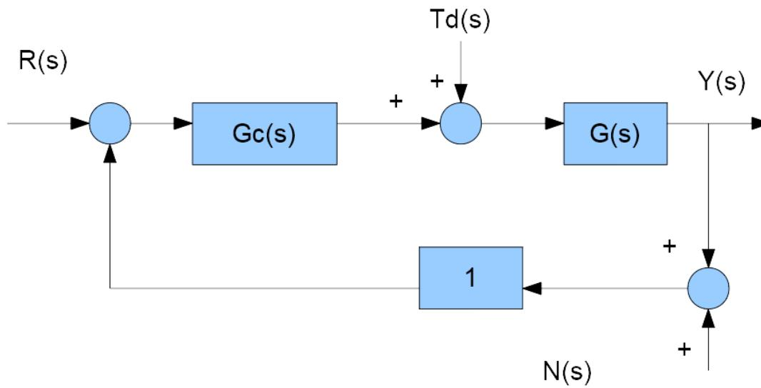
Inputs :  $R(s)$ ,  $Td(s)$  disturbance and  $N(s)$  measurement noise
