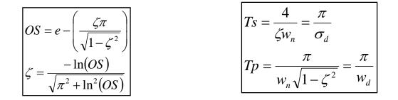
$w_d$  = damped frequency of oscillation  $\sigma_d$  = exponential damping frequency
