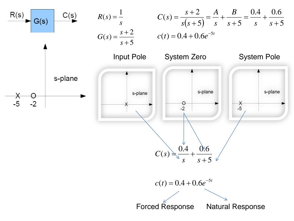
A pole of the input generates the *forced response* (pole at the origin generated from a step function at the output)
