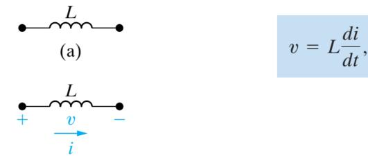
Voltage across the terminals of an inductor is proportional to the time rate of change of the current in the inductor.
