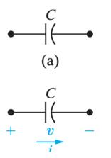
The circuit parameter of capacitance is represented by the letter C, is measured in farads (F), and is symbolized graphically by two short parallel conductive plates, as shown in Fig
