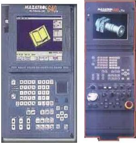
Mazatrol kontrol paneli
