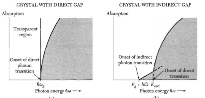
In (a) The threshold determines the energy gap, optical absorption is weaker near the threshold.
