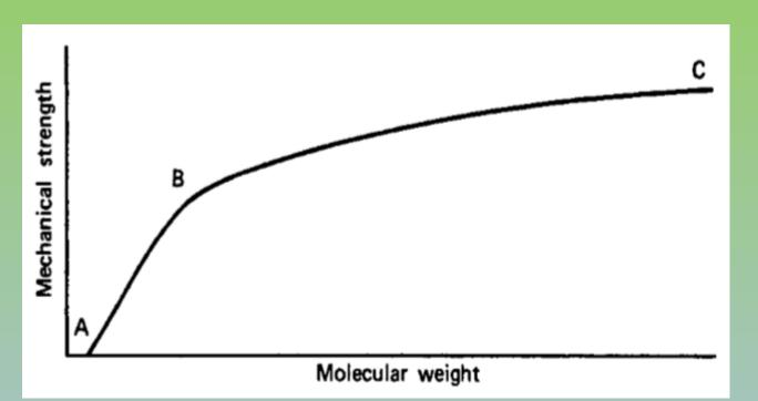
Figure shows dependence of mechanical strength on polymer molecular weight
