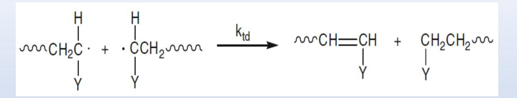
On the other hand, more rarely, they can be terminated by a disproportionation reaction, in which a hydrogen radical that is beta to one radical center is transferred to another radical center. This results in the formation of two polymer molecules—one saturated and one unsaturated as shown
