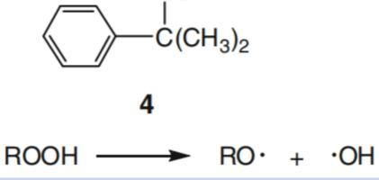
Hydroperoxides such as cumyl hydroperoxide 4 decompose to form alkoxy and hydroxyl radicals. Because hydroperoxides contain an active hydrogen atom, induced decomposition occurs readily, for example, by a chain-end radical. radicals may also combine Peroxy with subsequent formation of oxygen.
