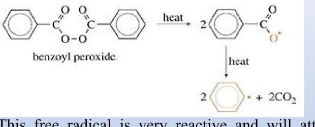
This is an unstable chemical which produces active species that attack the monomer. A good example is benzoyl peroxide which splits up when heated:
