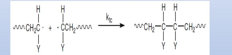
Two radicals are easily be terminated by a combination (coupling) reaction as shown
