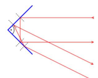
If the angle between two mirrors is 90°, the reflected beam returns to the source parallel to its original path. This phenomenon, called *retroreflection*, has many practical applications.
