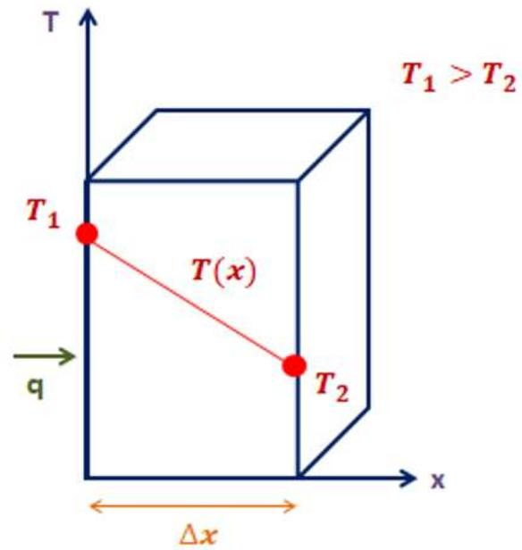
One-dimensional heat transfer by conduction (steady-state cond.)
