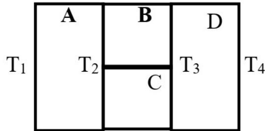
$$q = \frac{T_1 - T_4}{\frac{L_1}{k_A A_A} + \frac{1}{\frac{L_2}{k_B A_B} + \frac{L_3}{k_C A_C}} + \frac{L_3}{k_D A_D}}$$
