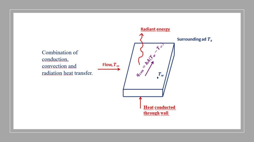
The heat conducted through the plate is removed from the plate surface by a combination of convection and radiation. An energy balance gives:
