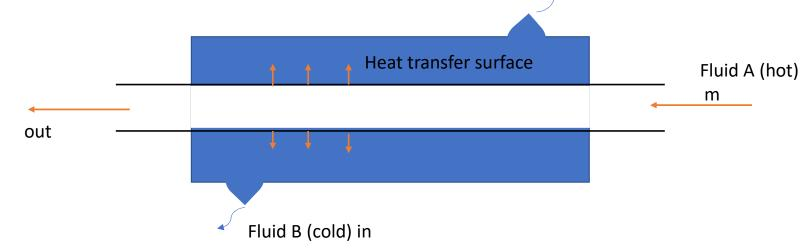
• Double-pipe exchangers are useful when not more than 100 to 500  $ft^2$  of surface area is required.
