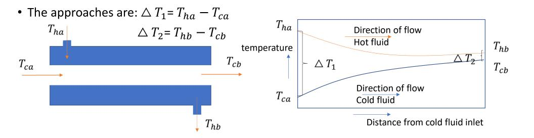
**Parallel flow:** Parallel flow is used in special situations that are:
