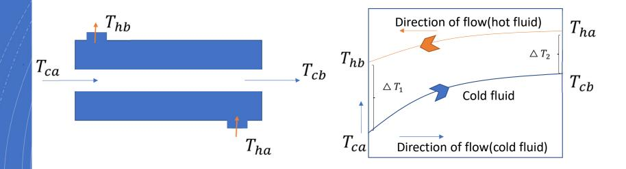
$T_{ha} \rightarrow temperature of entering hot fluid$   $T_{hb} \rightarrow temperature of leaving hot fluid$   $T_{ca} \rightarrow temperature of entering cold fluid$  $T_{cb} \rightarrow temperature of leaving cold fluid$
