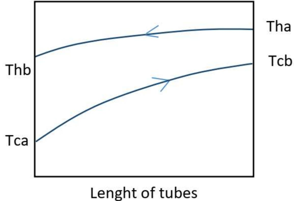
$$q = UAF_G \Delta \bar{T}_L = \dot{m}_c C p_c (T_{cb} - T_{ca})$$
