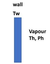
Condensation occurs when a vapour with the saturation temperature Th (such as steam) comes in contact with the surface, which is maintained at Tw; Tw is less than Th.
