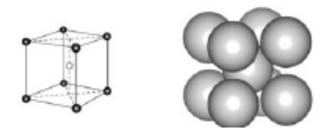
In body-centered cubic (bcc) structure, atoms contacting each other are seen on diagonals and then we obtain the following relationship:
