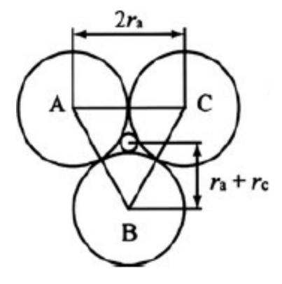
(1) When the coordination number is 3, a cation is likely to occupy the position equivalent to the center of an equilateral triangle of ABC formed by three anions as shown in Fig. 1. The height and the center of gravity for the equilateral triangle with its one edge being  $2r_a$  are given by  $\sqrt{3}r_a$  and the height  $\times \frac{2}{3}$ , respectively. Then, the value of  $\frac{2}{3} \times \sqrt{3}r_a$  is exactly equivalent to  $r_a + r_c$
