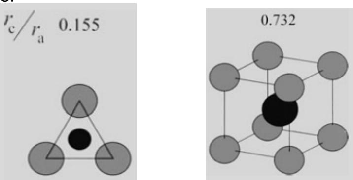
(1) When the coordination number is 3, a cation is likely to occupy the position equivalent to the center of an equilateral triangle of ABC formed by three anions as shown in Fig. 1. The height and the center of gravity for the equilateral triangle with its one edge being  $2r_a$  are given by  $\sqrt{3}r_a$  and the height  $\times \frac{2}{3}$ , respectively. Then, the value of  $\frac{2}{3} \times \sqrt{3}r_a$  is exactly equivalent to  $r_a + r_c$
