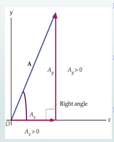
The x-component of a vector is the projection along the x-axis
