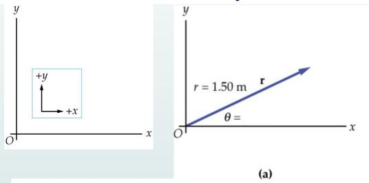
Vectors: Can be described by their magnitude and direction. For example: Your displacement is 1.5 m at an angle of 30°.
